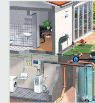
Rain Water Harvesting
